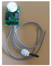
Left:- Usual replacement thermostat supply. All connected cables should usually be removed to facilitate easier connection to existing wires in thermostat end unit. No sensor has failed us in the last seven years!
